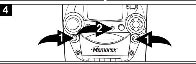
Adjust the MIC VOLUME control ① as desired. Increasing this control will increase the volume of the microphone. Adjust the ECHO control ② to add an echo effect to your voice. The ECHO control ② is variable so add as much or as little reverb as desired. Sing or talk into the microphone and you will hear both the CD+G and the microphone.
